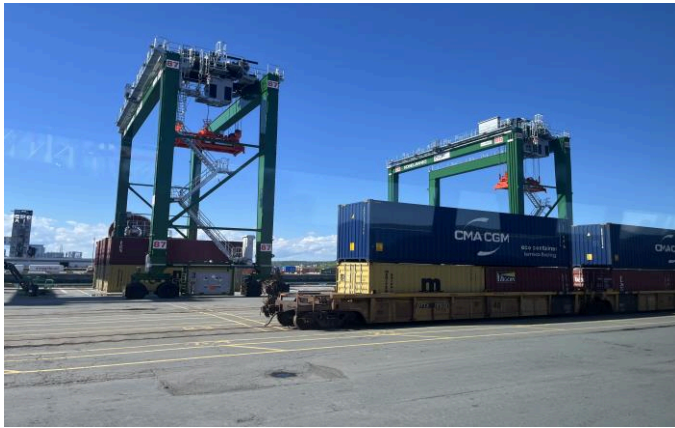
Exhibit 2: Port of Halifax's new electric rubber tyre gantry cranes (E-RTG)
