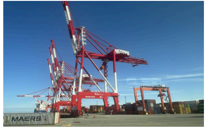
Exhibit 3: Port of Halifax's mega ship-to-shore (STS) vessel cranes
